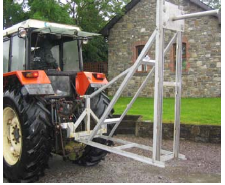
Figure 6. Mobile lance attached to tractor
